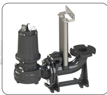
This is the most convenient solution for fixed installations, because the pump can be easily and quickly extracted and repositioned in the tank, meaning the pump can be serviced and cleaned without having to empty the tank or unbolt any parts.
